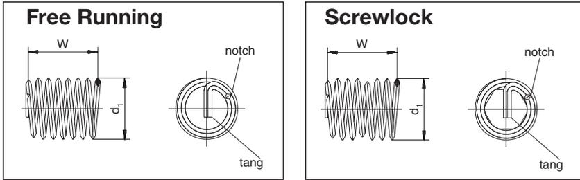
W and d<sub>1</sub> are the control values for thread inserts (Free Running and Screwlock) before they have been installed. The length can only be measured for installed thread inserts.
